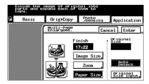
15 Using the keypad, type in the desired zoom ratio, and then touch [Enter].
